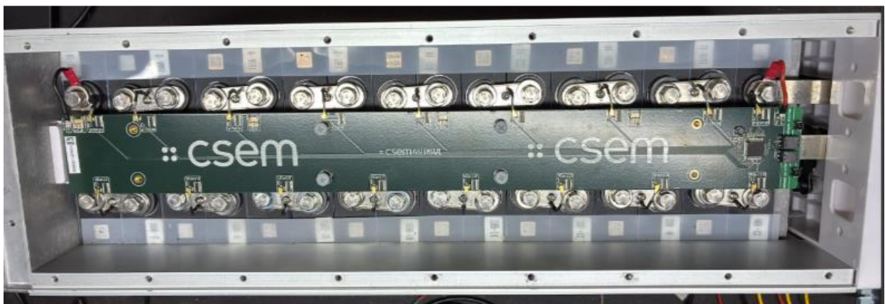
Figure 1: module level slave board with EIS sensing capabilities
